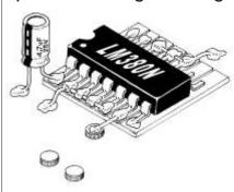
Construction of LM380 pins 8-14
