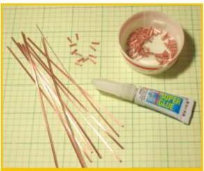
Fig. 3 – The basics for *Manhattan-031*. Strips of .031 copper clad are cut into narrow strips with a PCB shear or regular scissors; pads were made with a nibbling tool; super glue is used to affix the pads and strips to the main copper clad board.
