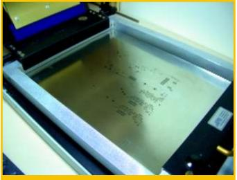
FIG. 24 – A stencil mounted, ready for pasting
