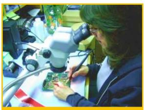
Fig. 8 – Connie Angel, one of the professional assemblers at the VLA observatory, solders surface mount components onto a board with tweezers and a soldering iron. The board is part of a new radio telescope (called ALMA) being built in Chile.
