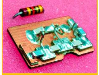
FIG. 16 – A 1090 MHz High Pass Filter made from SMC capacitors and "hand made" inductors Manhattan-031 style.
