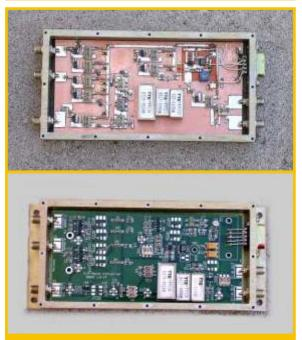
FIG. 19 – The Manhattan-031 prototype VHF upconverter (top) became the model for the PCB (bottom) with few differences, and mounted inside RFI enclosures.
