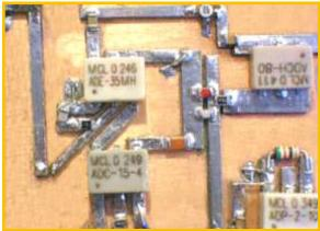
Fig. 4 – The strips form "traces" similar to a PCB for orderly mounting of the SM components. Often, diagonal runs will be more convenient, as shown here.
