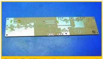
FIG. 25 – The PCB "pasted" with the above stencil. This board down-converts the VLA 8–12 GHz IF to 0–4 GHz baseband, then digitally sampled at 8 GHz.
