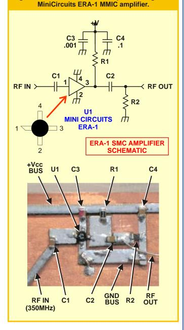
The pads, islands and strips were cut from .031" copper clad. The main board, in this case, was also .031, although either .031" or .062" could be used. The pads and strips were affixed with super glue.
