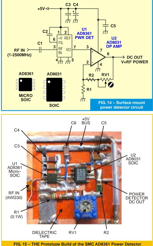
The Micro-SOIC package is just too small to properly build on a prototype level without a microscope. The other surface mount IC, the U2 AD8031, in the "normal" SOIC package, was relatively painless. The rest of the circuit was built in a fairly straightforward way – mounting the SMC components between .031" Manhattan pads.
