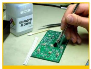
Fig. 9 – Clean solder connections with a hobby brush and alcohol. This keeps the board clean and free of corrosive rosin, whether building Manhattan or a PCB.
