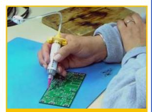
Fig. 22 – A closer view of the solder paste syringe. Air pressure deposits extremely small drops of paste of uniform size.
