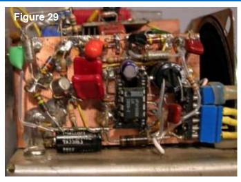
The AM detector and audio amplifier portion of a shortwave receiver built "ugly" style. The unused endpins of the IC socket are soldered to the copper clad. The remaining socket pins are bent outward to make the connections.
