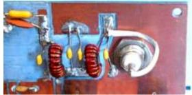
The PA Output Filter mountedon the inside of the rear panel saves space
