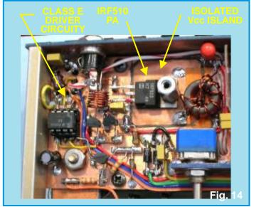
A closer view of the transmitter section, showing the Manhattan style of construction.
