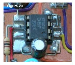
The LM386 Audio Output Amplifier IC
