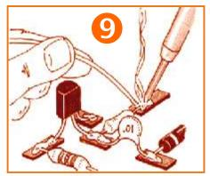
The glued pads become mounting platforms for the components, soldered in place.
