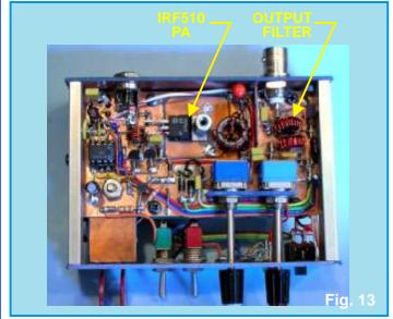
Bottom view of the Rockmite, showing the home-brew transmitter section built Manhattan Style.
