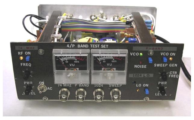
Most parts came from Mouser or MiniCircuits. The copper clad, meters and a few other parts were purchased from Electronic Goldmine. The rest of the parts were lab stock or what could be scrounged around the lab. Metal work was cut, bent, drilled and milled in our own model shop. I used copper clad pads made from a nibbling tool for the most part, or long, narrow strips for Vcc runs, etc.
