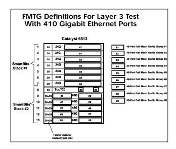
The diagram on this page shows the nine groups of 48port Full Mesh Traffic Groups (FMTGs) used in this test and illustrates that traffic was switched both locally and across the fabric between cards.As with the previous L2 performance tests, we adopted two test configurations, the worstcase configuration shown in the diagram above and a best-case configuration where all traffic stayed local to each card.
