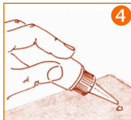
Pads are "mounted" to the main circuit board with glue – usually with super glue. The secret is learning to administer a small drop of glue. This comes with practice.
