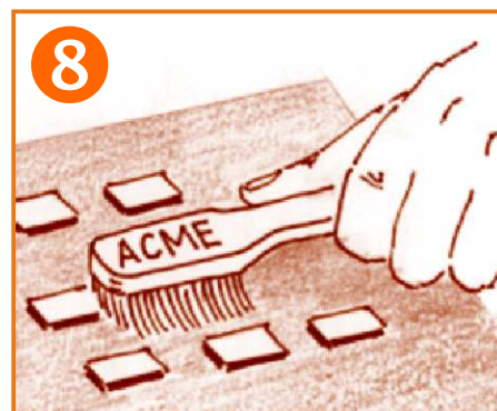
Clean board and pads with a brush and alcohol or acetone.
