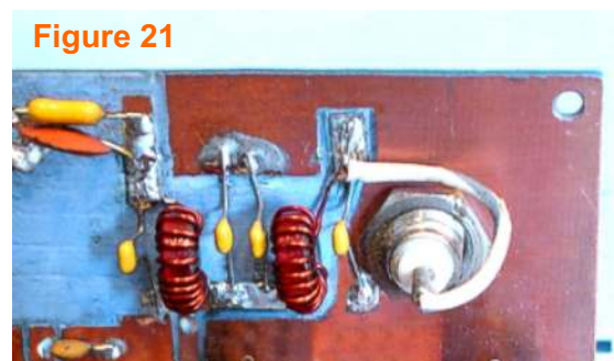
The PA Output Filter mounted on the inside of the rear panel saves space
