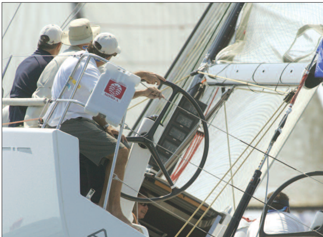
The mast is a great place to mount your boatspeed readout (and other important instruments) because it's easy to see the numbers while looking forward. That way you can simultaneously watch the instruments, telltales, waves and angle of heel. You wouldn't want to use instruments that are mounted in the cockpit because you'd have to look down to see them and that would interrupt your view of everything else.
